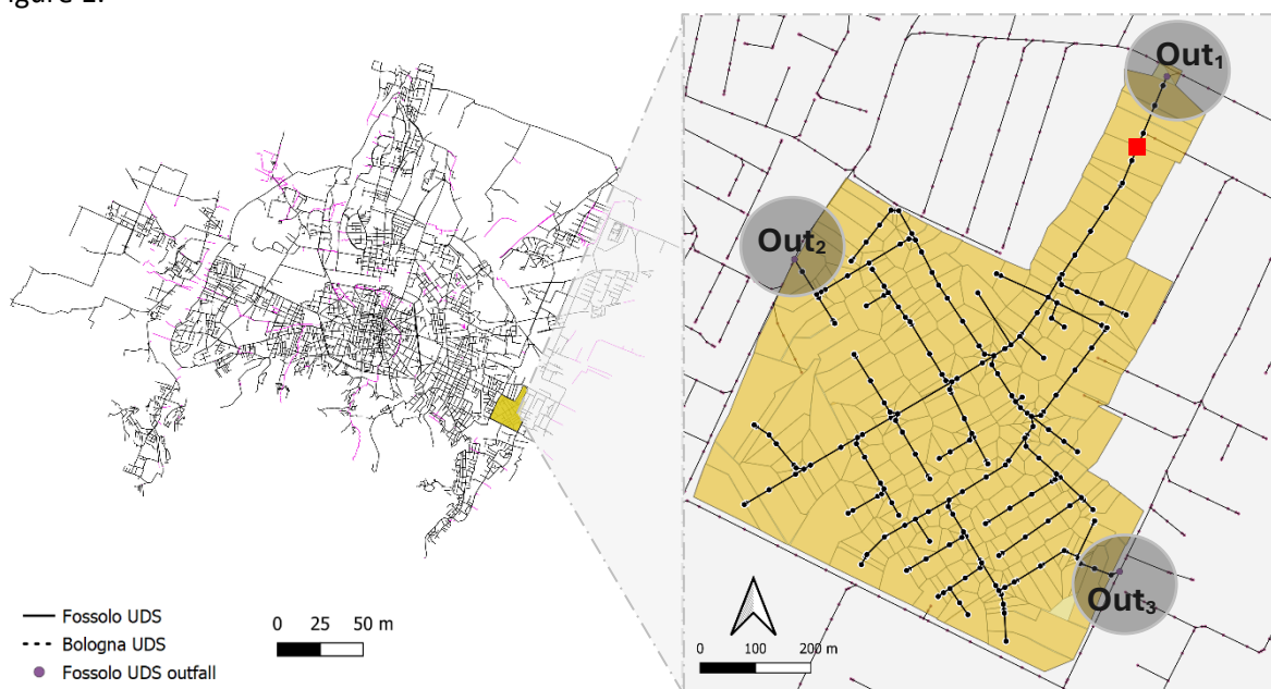
Figure 1. Bologna sewer network with a focus over Fossolo catchment and relative drainage system and outfalls. Red square represents the location of the water level sensor.
