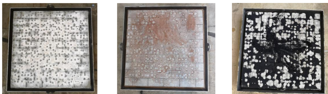
Figure 2.: Milisill W4 mineral dust (left), road dust sediments collected from UDC parking lots with a realistic (non-uniform) PSD (center) and plastic tyre dust at IKT test stand (right) during the experimental campaign on ICBP pavement.
